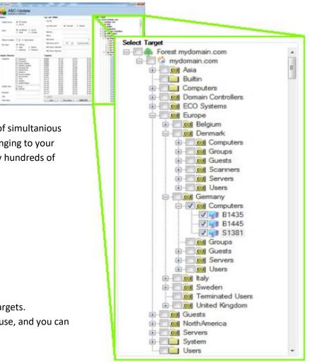
Or click the "input" button to write name of targets. Named targets can be saved to a file for later use, and you can read targets from files.
